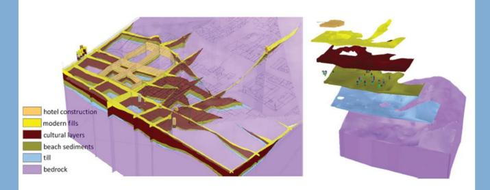
Modell of layers in the subsurface below Bryggen. The cultural layers, consisting mostly of organic material from human waste, can be more than 10 meter thick. Underneath are natural sediments beposited by the fjord and glacier, on top of bedrock. The walls of the modern hotel, sheet pile wall, is marked with orange in the modell (Source: De Beer, 2015).
