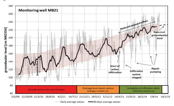
Groundwater level in monitoring well MB 21. The grey line shows daily variations of the groundwater level. The black curve gives a simplified impression of the groundwater level, by showing average values over three-month intervals. Graph: Anna Seither, Geological Survey of Norway
