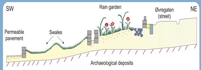
Section of the sustainable water management "treatment train", with rainwater garden, swales and permeable pavement. Drawing: Johannes de Beer, Geological Survey of Norway.
